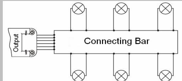
When distance between transformer and halogen lamps is big use conection as shown below, don't use series connection.
