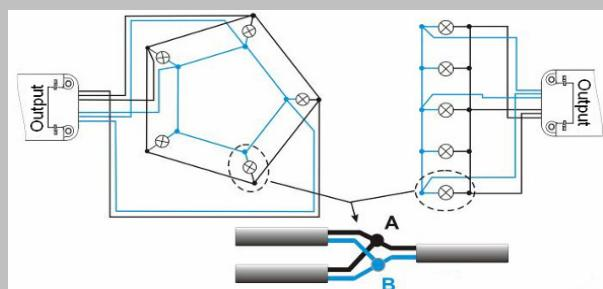
Load on pair of output terminals cannot exceed 85W. Load should be divided equally on all output terminals.
